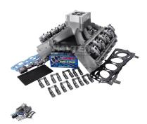
TOP END KIT- SBC Street Solid Roller Cam/ Alloy Heads/ Single Plane Intake (655 HP)
