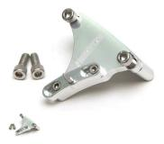
SBC 6-1/4" TIMING POINTER SILVER WITH 4 DEG OF ADJUSTMENT
