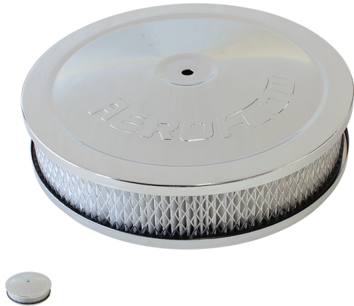
Chrome Air Filter Assembly 9" x 2", 5-1/8" neck, paper element
