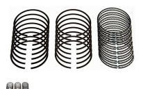
Plasma Moly V8 Ring Set. 4.030 Bore, 1/16" X 1/16" X 1/8", Std Tension. Not Filebacks
